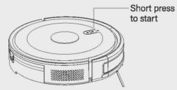
Please install the side brush and lock the screw before use. Remove the foamblock next to the bumper.
